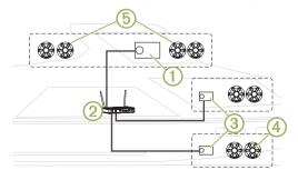
In the image above, one Apollo RA670 stereo ① connects to a wireless router ② and to two Apollo SRX400 zone stereos ③. A FUSION PartyBus zone stereo, such as the Apollo SRX400, controls the volume in a single speaker zone ④. A FUSION PartyBus stereo, such as an Apollo RA670 stereo, controls the
