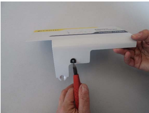
c. Adjust and insert the protective seal
