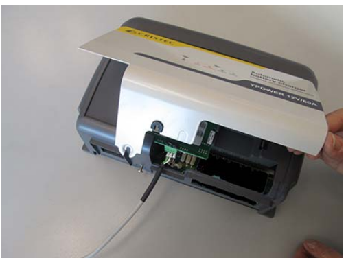
d. Put the charger clasp back in place and use this opening to get the cable through.
